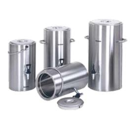
CE - series: equipped with a heating element with klixon thermostat that does not touch the bottom. This gives a hot air au bain-marie effect that maintains the proper temperature of the beverage (about 85 °C) and it can be kept for a longer time. Options: 4, 6, 8, 10, 12, 16, 20 or 25 litres. 4 - 8 litre containers have a carrying bracket, the others have grips.
