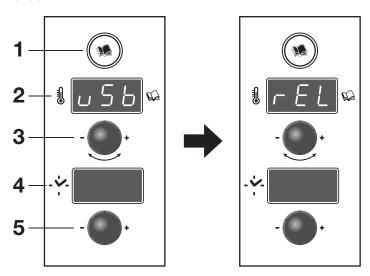
With the appliance live and display off, press button 1, the display 2 shows [USb], turn knob 3 until [rEL] is displayed, press the knob to confirm the selection
